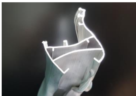
Figure 1. Product defects with an improper extrusion die design. The defects concern with significant bending and twisting of the profile.
