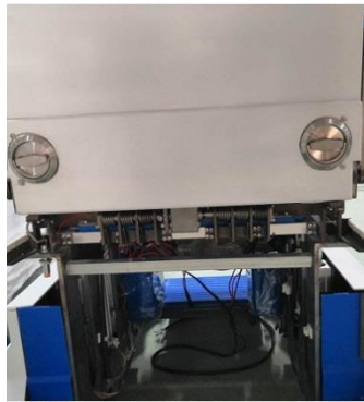
Figure 24. The driving device of folding mechanism.
