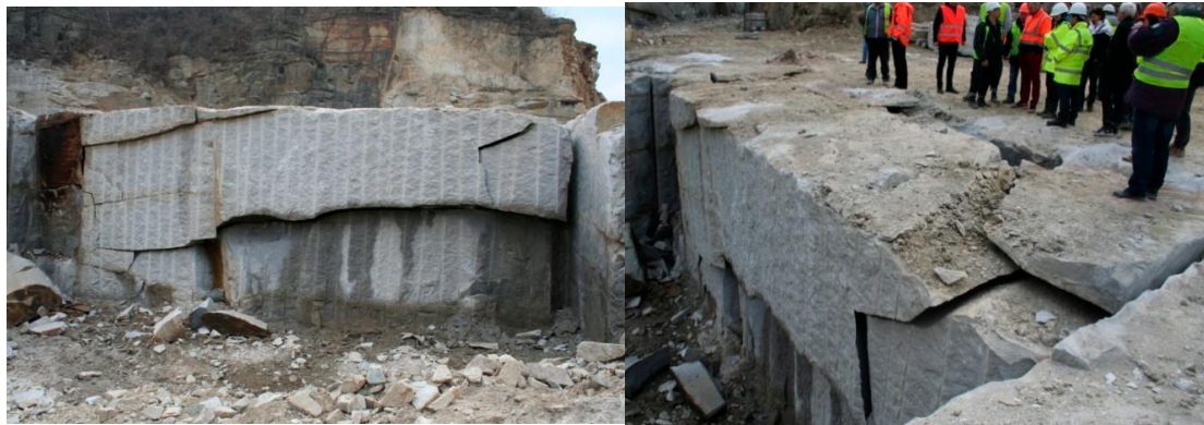
Figure 9. The effect of RSP in a granite deposit.
