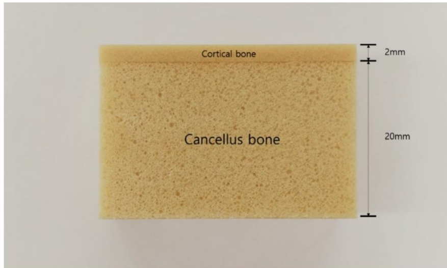
Figure 2. Digital photograph of a artificial bone block.
