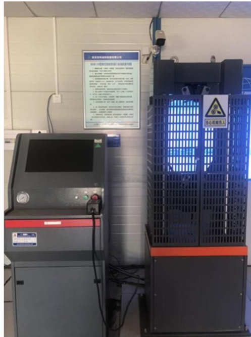
Figure 2. WAW-100 hydraulic servo universal testing machine. Figure 2. WAW-100 hydraulic servo universal testing machine.
