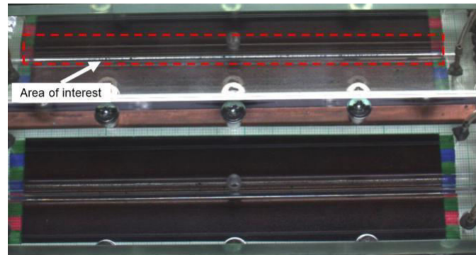
Figure 5: Actual frame taken by the camera in not a perpendicular (tilted) position.
